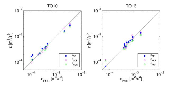
Figure 1: Dissipation rate of the kinetic energy estimated from the structure function method  $\epsilon_{SF}$ , zero-crossings of successively filtered signals  $\epsilon_{NCF}$  and zero-crossings of signals with recovered part of the spectrum  $\epsilon_{NCR}$  as a function of  $\epsilon_{PSD}$  (from power spectra method). Each point represents a single segment of flight from POST campaign [2], a) flight 10, b) flight 13.
