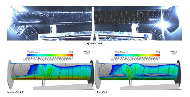
Figure 1: Comparison of oil and mini-tufts visualisation with numerical results of wall-shear
