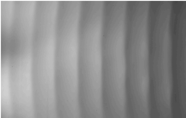
Wave propagation for a flat bottom and the frequency f = 2.8 Hz
