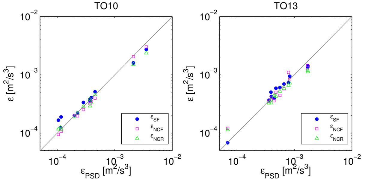
Figure 1: Dissipation rate of the kinetic energy estimated from the structure function method  $\epsilon_{SF}$ , zero-crossings of successively filtered signals  $\epsilon_{NCF}$  and zero-crossings of signals with recovered part of the spectrum  $\epsilon_{NCR}$  as a function of  $\epsilon_{PSD}$  (from power spectra method). Each point represents a single segment of flight from POST campaign [2], a) flight 10, b) flight 13.
