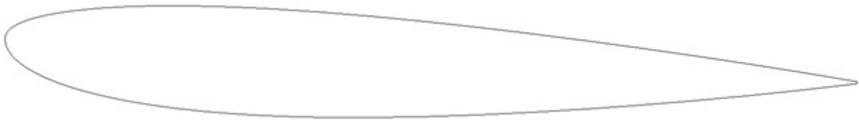
Figure 1: Airfoil m1510 set at a 3 degrees angle
