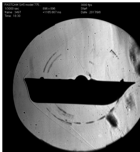
Figure 2: Visualization of flow around wrap-around fin, \alpha = 1^\circ , Mach = 1.9
